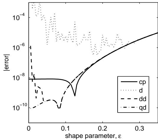
Figure 9: Standard and extended precision Gaussian Elimination and Contour-Padé error versus the shape parameter for approximating  $\partial f / \partial x$  of function  $f(x, y) = \exp(x/2 + y/4)$  at the point  $(0.74874, -0.11558)$  that is marked in figure 8.
